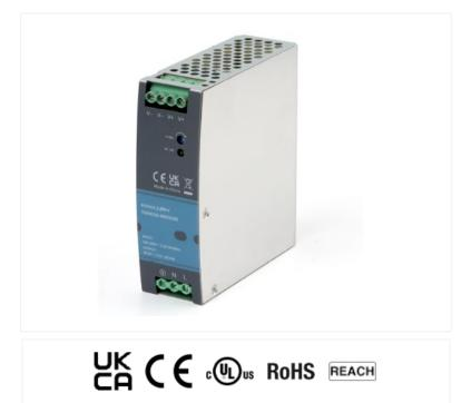
The 56YSDN75-xy Series is a high-performance 75W DIN Rail Mount AC/DC Power Supply. Designed for use in applications such as digital signage, displays and user interfaces. This series is supplied with a Screw Terminal Block input connection and supports input voltages of 90~264V AC 50~60Hz.
